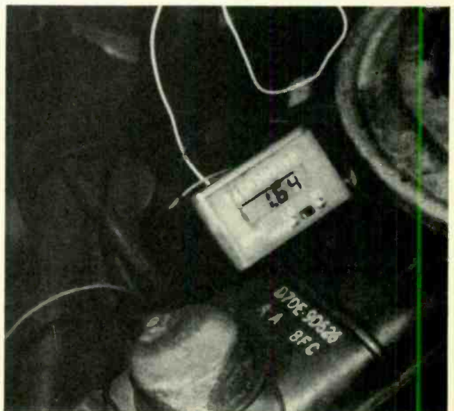
EVEN IN THE DIM LIGHT in the engine compartment of this old Ford, the Digital AutoTach liquid-crystal display clearly indicates the engine's rpm . The unit shown was constructed as an outboard tester for tune-ups.
